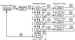
Figure 4. Flow chart of how to set the alarm
