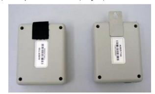
Figure 6. Left, using Velcro for mounting. Right, using stainless steel plate for mounting.
