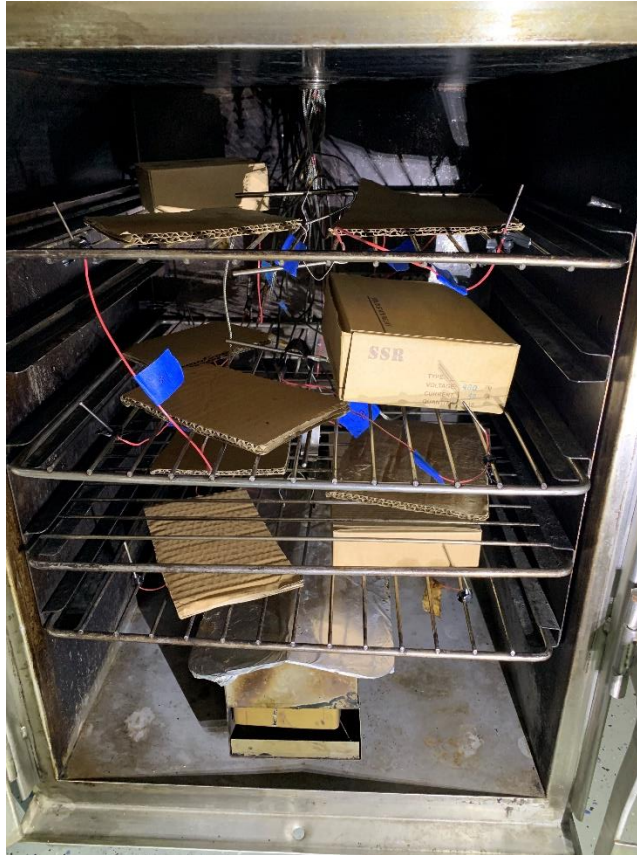
Figure 2. Cardboard boxes and cardboard sheet of different size that were selected and randomly placed in the smoker to simulate different food chunks.
