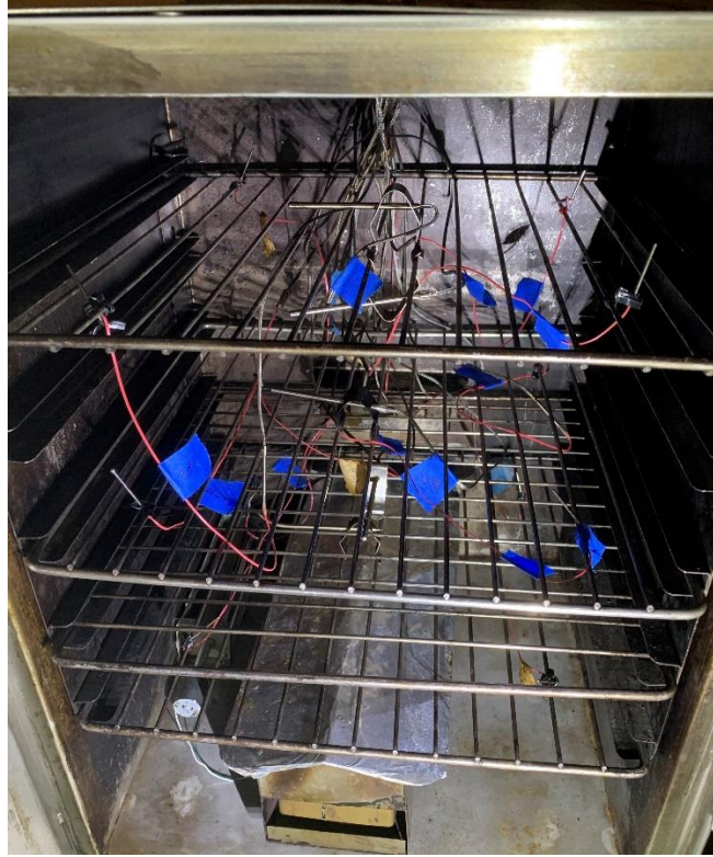
Figure 1. total 17 temperature probes were installed on this testing smoker.
