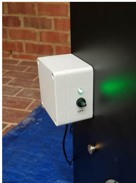
Figure 22. Flip the toggle switch up to turn on the fan.
