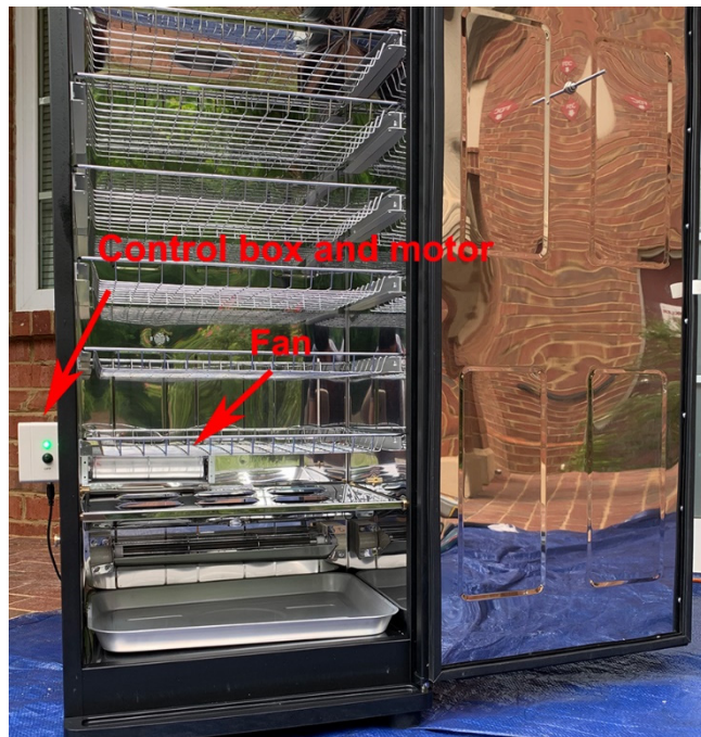
Figure 11. The CIRFAN kit installed on a smoker.
