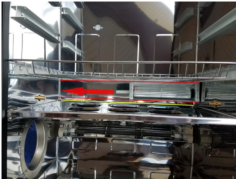
Figure 12. Check if there is enough space for installing the fan.
