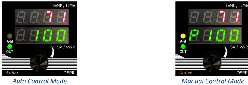
Figure 3. Compare the differences of the display on a DSPR-5 in Auto Control Mode with the SV set at 100°F (left) and the controller in Manual Control Mode with the SV set at 100% output (right).
