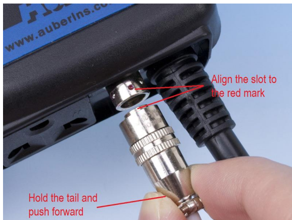
Figure 3. Install the Sensor.
