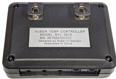
Figure 10. Two mounting hooks installed on the back of a SYL-3615 controller.
