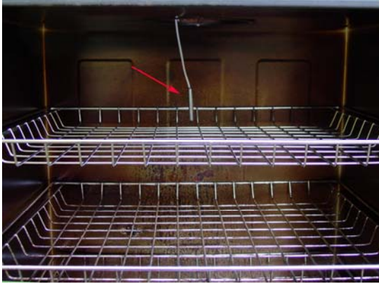
Fig 5. Sensor position. Left, the sensor should be placed close to the food but high enough so that it does not touch the food. Right, hold the sensor in place by a piece of tape.
