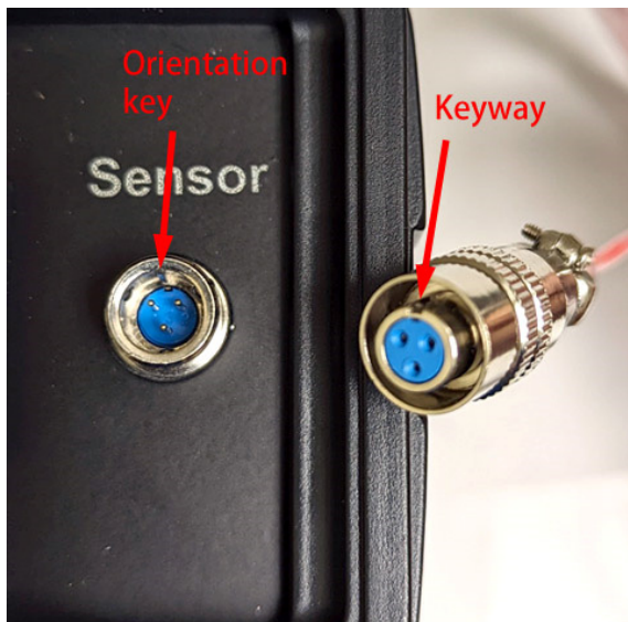
Figure 3. Orientate the sensor plug to match the sensor socket on the controller.
