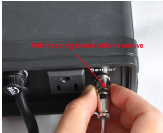
Figure 4. Pull the spring-loaded collar to remove the sensor.
