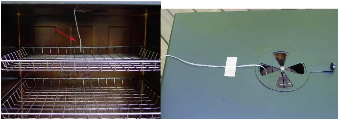
Figure 3. Sensor position. Left, the sensor should be placed close to the food but high enough so that it does not touch the food. Right, hold the sensor in place by a piece of tape.
